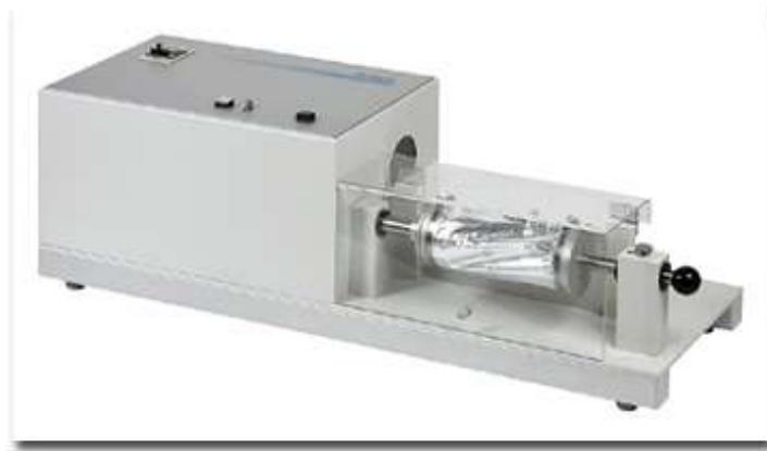
The apparatus is used for simulating a creasing strain of flexible packaging materials (KFT).
