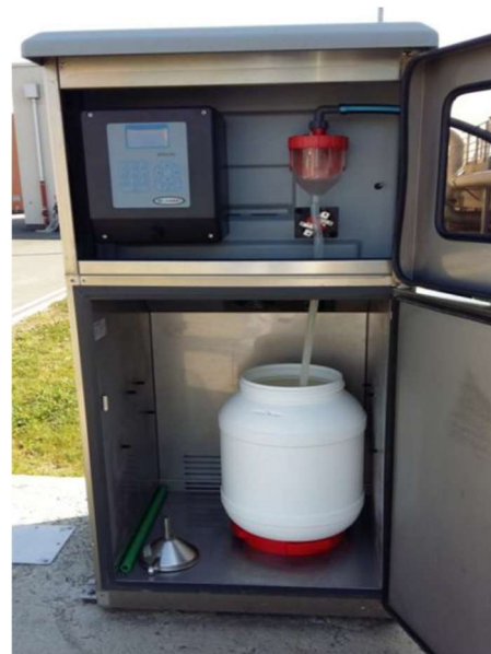
Figure 3. Automatic sampler for influent
