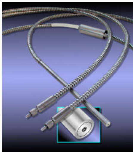
Figure 2: reflection probe with 6 illumination fibres and one reading fibre which can be connected to the spectrometer
